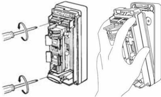
The battery must be disconnected before SIM card installation or removal. Insert the SIM card into the exposed SIM holder and refit the back box ensuring that the battery is refitted in the padded section of the housing above the electronics.
